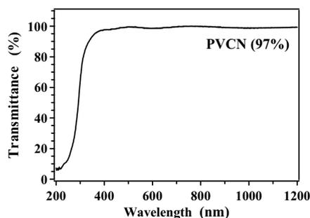
Fig. 2. Transmittance of PVCN-2.
